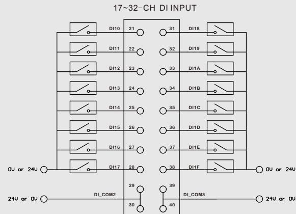
Terminals 29 and 30 are internally connected
