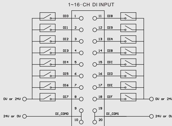
Terminals 9 and 10 are internally connected
